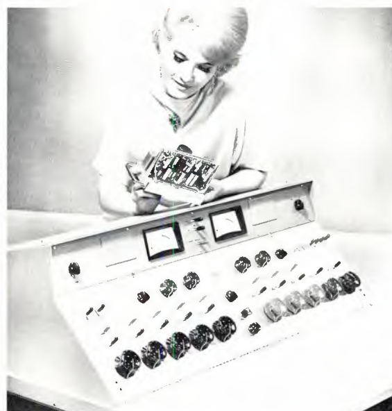
Plug-in chassis give flexibility to consolettes.
